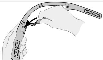
Take HEADBAND FRAME, insert forehead strap into center curved slot. TIP: Curved slots adjust nose-to-shield distance. 3 settings available.
